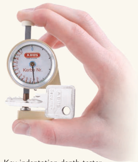
Key indentation depth tester on the basis of DM 2
