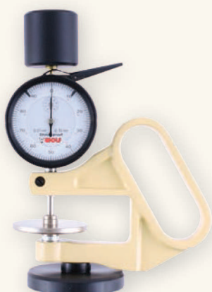
DMH 3-L especially for leather with a standardised gauging pressure of 50 kPa
