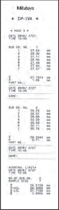
Mode 3 N: Number of data MAX: Maximum value MIN: Minimum value n: Number of subgroup (Max.10) X: Average value of subgroup R: Range of subgroup X: Mean value X-UC: Upper control limit R: Mean (R control) R-UC: Upper control limit (R control) R-LCL: Lower control limit (R control)
